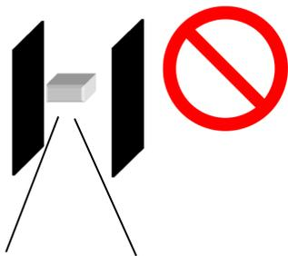
**Poor location:** Narrow window for detection. The signal can't be seen
