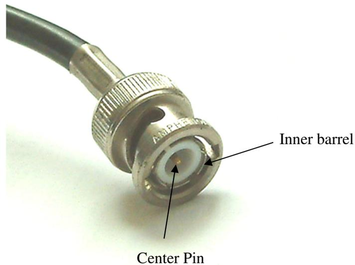
Make sure the center pin and inner barrel are flush on both ends of the cable. This is often the source of low hit numbers.
