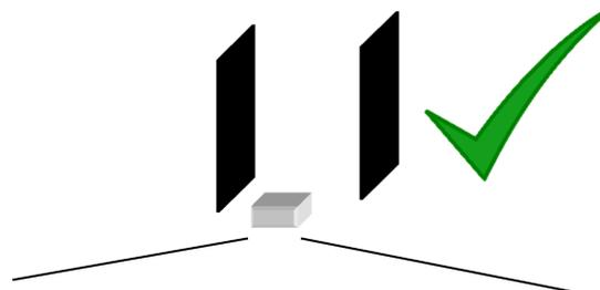
**Good location:** No metal to block the signal. The detection window is very wide.
